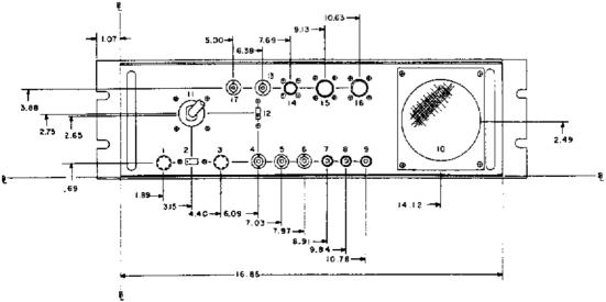
Figure 2-1. WJ-8888 Receiver, Critical Dimensions
